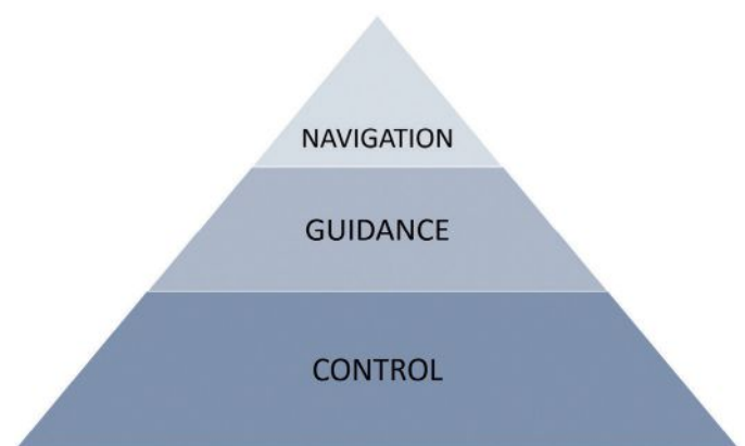
Figure 2. The vehicle operation primacy triangle displays how tasks of increasing primacy and consistent workload form the foundation for tasks of increasing complexity.
